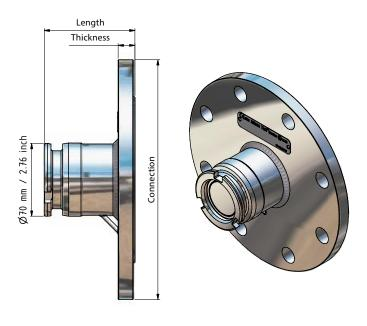
Example: 2" (Ø 70 mm) tank unit (adapter) with flange 4" ANSI 150 psi, Code No: T263A4401
