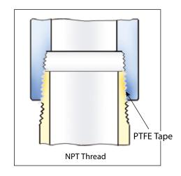
9. For extremely stubborn to seal threads, apply a normal coating of thread paste followed by a single layer of gauze bandage followed by a normal layer of thread tape.
