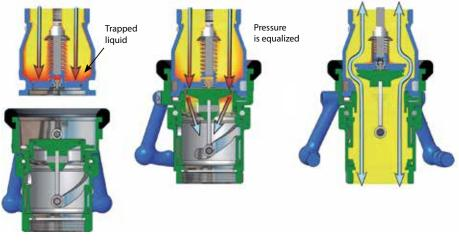
Trapped liquid in tank unit (above)
