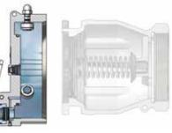
Pressure Indicator (warns for overpressure)
